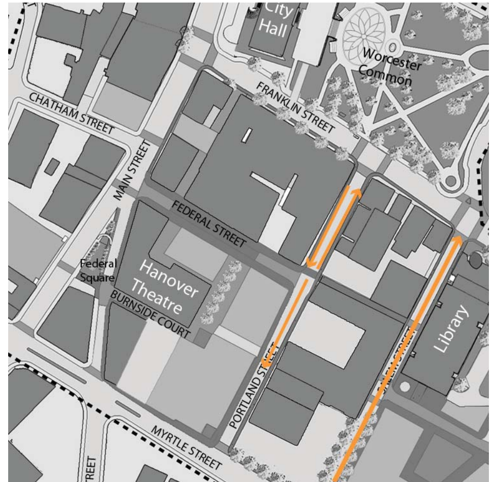
Proposed traffic flow on Portland and Salem Streets after introduction of angled parking.
