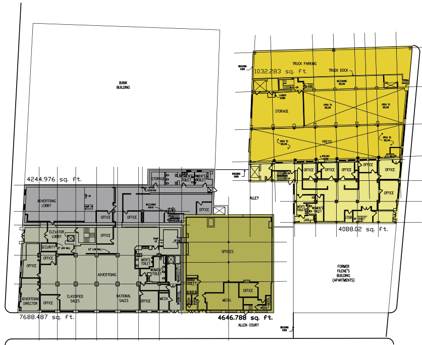
20 Franklin Street: existing ground level plan showing the five buildings that make up the property today. Plan courtesy of Cutler Design and the WBDC.
